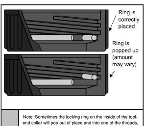
Note: Sometimes the locking ring on the inside of the toolend collar will pop out of place and into one of the threads, preventing the collar from closing all the way. If this happens, the tools will fall out and the collar wont tighten all the way. Push the ring down and out of the threads to remedy. When properly placed and the collar is tightened, the two ends of the rings should touch each other. Above is a cutaway illustration of the collar.
