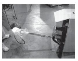
Secure the handle release lock. Tip the side of the carton where the wheels are located on its side and roll the machine out of the carton.
