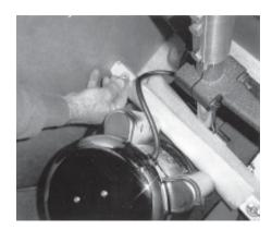
8. Remove wing nuts and washers to unfasten wood shipping retainer. Discard wood shipping retainer.
