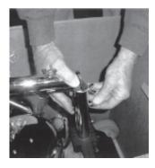
Remove the wing nuts and bolts from both upper and lower handle. Discard the angle bracket.
