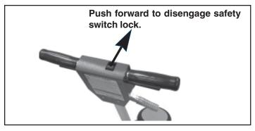
To stop the machine, simply release the triggers. The safety switch lock will automatically return to the engaged position.
