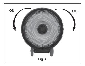
To install a brush or pad driver, leave the handle in the upright position and tip the machine backwards so it rests on its wheels and upper handle section (Fig. 4). The brush and pad driver both attach in the same manner: align the cutouts on the inner ring of the brush or pad driver with the tabs on the inside of the ring of the drive hub (Fig. 5). Push the brush or pad driver firmly in position, then turn it counterclockwise until it locks into place.
